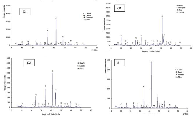
Fig.1: Diffractometer diagram of aggregate used.
