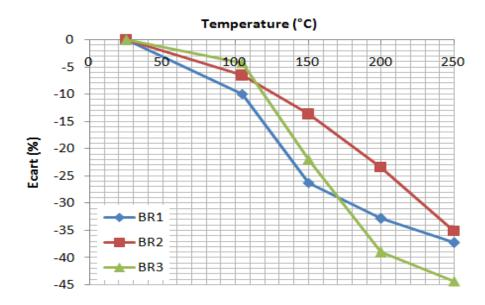
Fig. 3. Evolution of the ecart of thermal conductivity of concretes tested as a function of temperature
