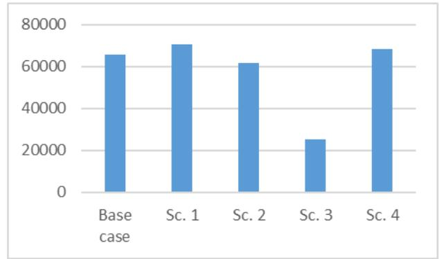
**Fig. 5.** Comparison of annual total heating loads [kWh] for all scenarios.
