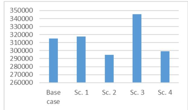
**Fig. 6.** Comparison of annual total cooling loads [kWh] for all scenarios.
