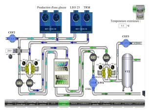
Fig. 13. Cooling system BMS diagram
