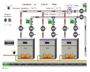
Fig. 5. Heating system diagram - boilers
