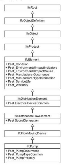
**Fig. 2.** Possible Pset collections of the pump in connection with the inheritance hierarchy of the IFC model
