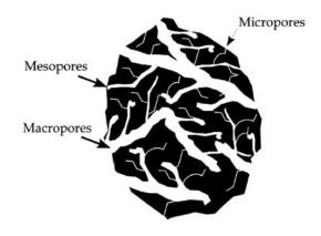
Fig. 1. Schematic representation of adsorbent pore structure [14]
