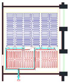
Fig. 3. Layout of the radiant ceiling system.
