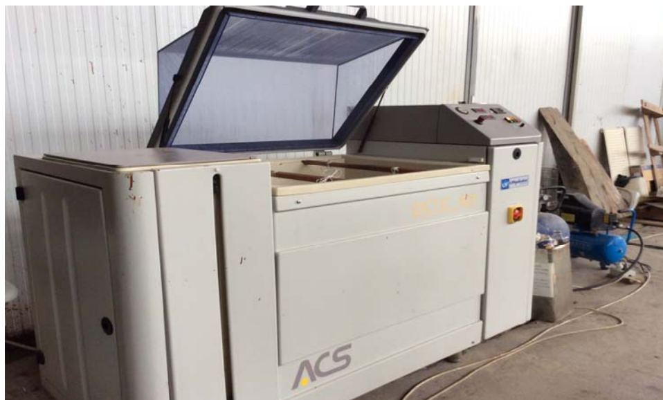
Foto nr.12 "Camera climatică" Dry Corrosion Test Cabinet (DCTC)600 fabricat de Angeloantoni Industrie
