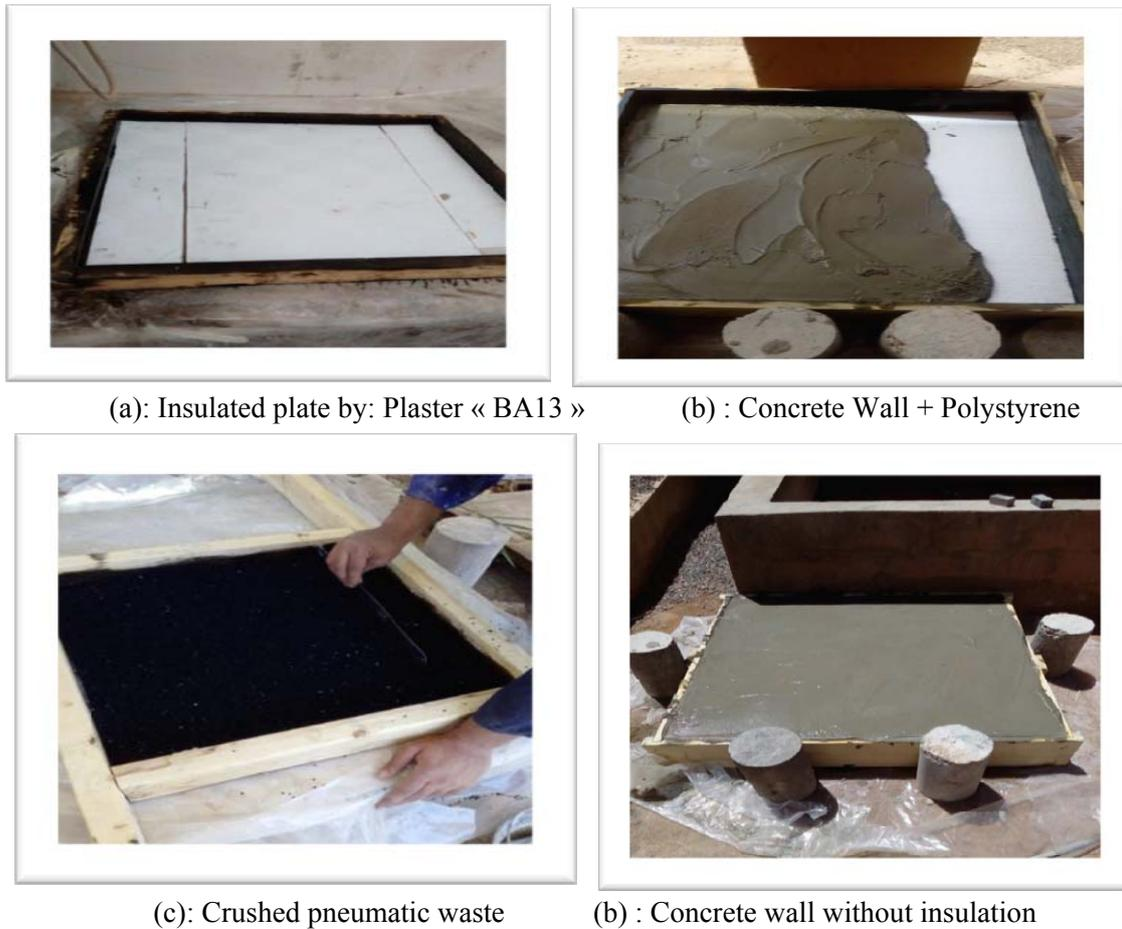
Fig. 4: Test specimens.
