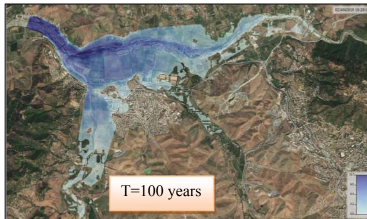
Figure 5. Floodplains obtained for events with return periods (T10; T25; T50; and T100 years) flow rate on the project area. source: own elaboration
