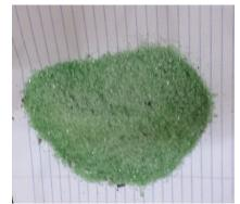
Plate 1. Sample of the recycled glass powder used in the study
