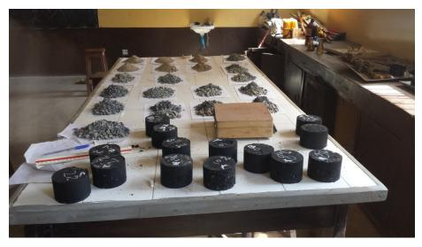
Plate 3. Air curing of the asphalt samples
