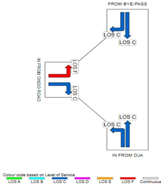
Fig. 7. LOS on each leg at Bye-pass intersection
