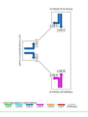
Fig. 5. LOS on each leg at Bye-pass intersection
