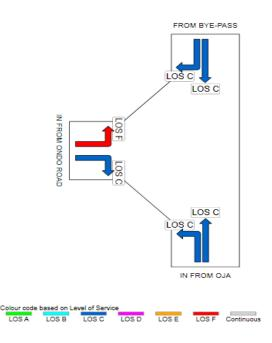
Fig. 7. LOS on each leg at Bye-pass intersection
