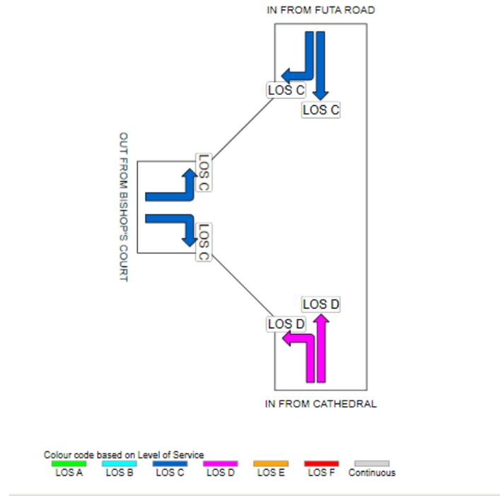
Fig. 5. LOS on each leg at Bye-pass intersection
