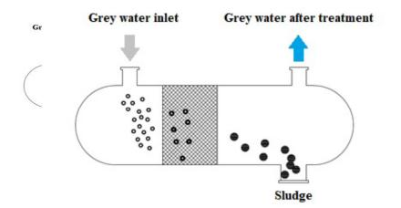
Figure 2: Schematic illustration of a horizontal coalescence filter
