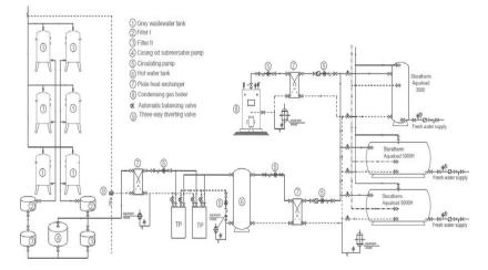
Figure 8: Proposed hydraulic scheme of DHW system with a GWW as a source of heat
