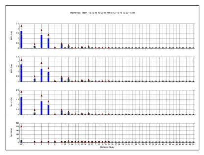
Figure 2. Harmonic spectrum of currents on the three phases and zero
