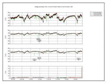
Figure 1. Variation of voltages on the three phases and on the null
