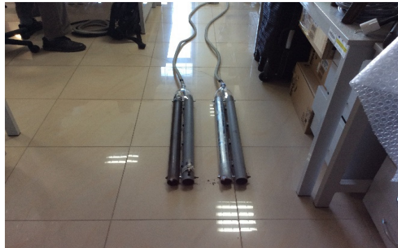
Fig. 5 Non-galvanized and galvanized metal samples with sensors
