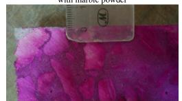
Fig.6. Determination of Carbonation depth with phenolphthalein pulverisation
