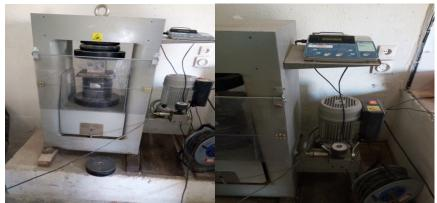
Fig.2. Machine for compressive strength test.
