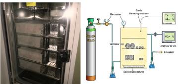
Fig.3. Accelerated carbonation chamber
