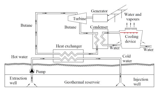
Fig. 1. Binary cycle geothermal power plant.
