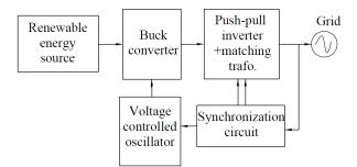
Fig. 3. Block diagram of the conversion system.
