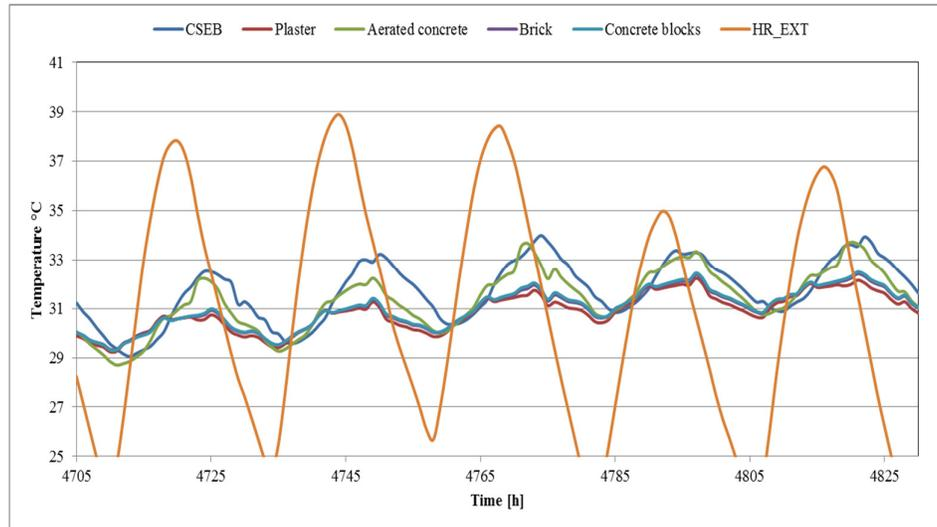
Fig.7. Interior temperature of zone Z1 of the ground floor apartment for the different materials tested during 5 days in July
