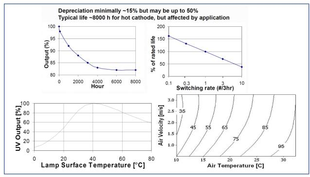
Figure 7 UV output change [%] with different parameters [10,16]
