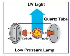
Figure 5 main operating principle of a UV-C lamp [8]
