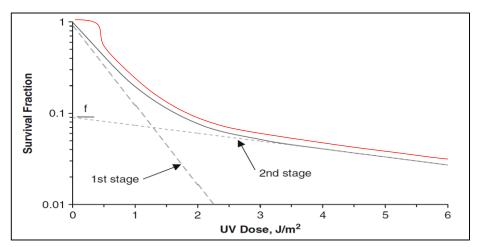
Figure 3 two-stage inactivation curve [adapted by CL from 6]
