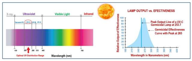
Figure 1 – electromagnetic spectrum and germicidal effectiveness of a UV lamp
