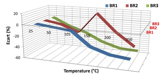
Fig. 3. Evolution of the ecart of thermal conductivity of concretes tested as a function of temperature
