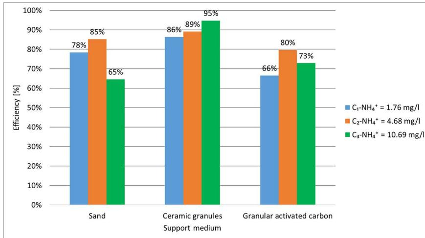
**Figure 3.** Biofilter efficiency of reducing the ammonium concentration depending on the filtration media used and the ammonium concentration in the raw water introduced in the biofilters - phase I.
