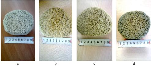
Fig. 2. Appearance of the cellular glass products a – variant 1; b – variant 2; c – variant 3; d – variant 4
