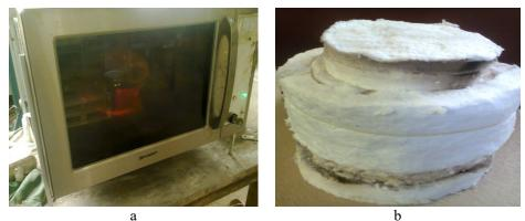
Fig. 1. Images of the experimental equipment a – adapted 800 W-microwave oven; b – ceramic fiber thermal insulation of the Y<sub>2</sub>O<sub>3</sub> coated crucible.
