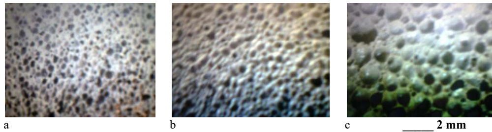
Fig. 3. Microstructural configuration of glass foam specimens a – specimen 1; b – specimen 2; c – specimen 3.
