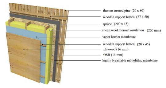
Fig.2. The constructive structure of the external walls
