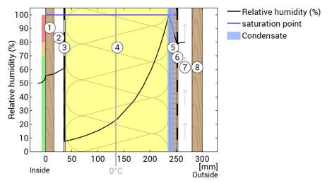
Fig.5. The relative humidity inside the component
