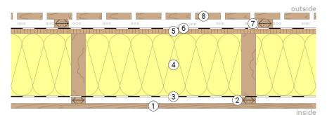
Fig.3. Section through the exterior wall
