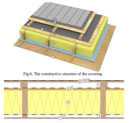
Fig.7. Section through the roof
