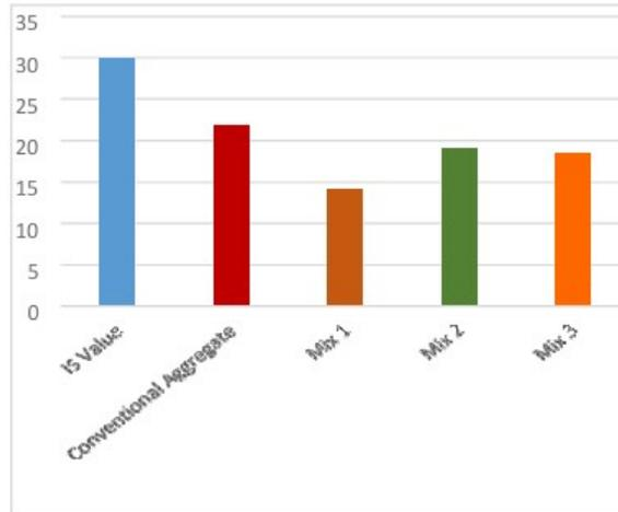
The crushing value is an important property of aggregates, representing their resistance to crushing under a gradually applied compressive load. It helps assess the quality and suitability of aggregates for use in construction, especially in high-load-bearing applications. Comparison of Crushing Value for Conventional and Lightweight Aggregates. Conventional Coarse Aggregates typically consists of materials like crushed granite, basalt, or natural gravel.
