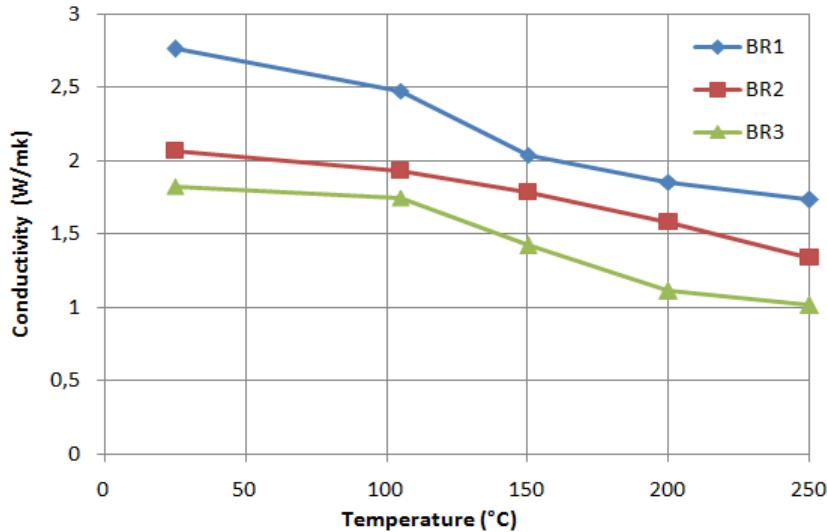
Fig. 2. Evolution of the thermal conductivity of concretes tested as a function of temperature
