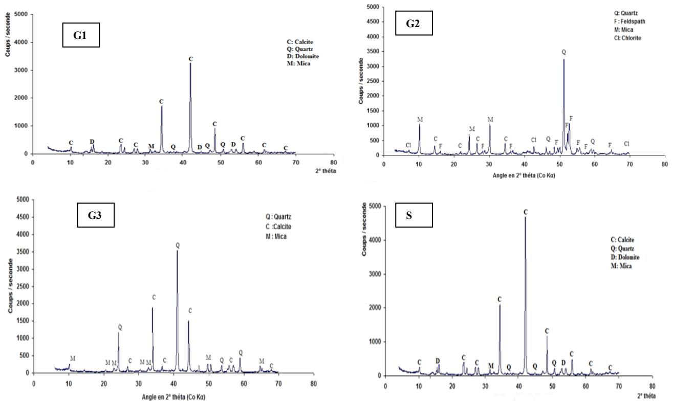
Fig.1: Diffractometer diagram of aggregate used.
