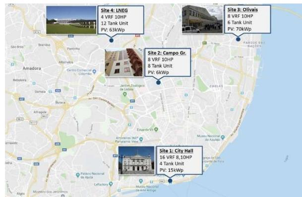
Figure 1. Installation of AC and PV systems in four buildings in the city of Lisbon, Portugal
