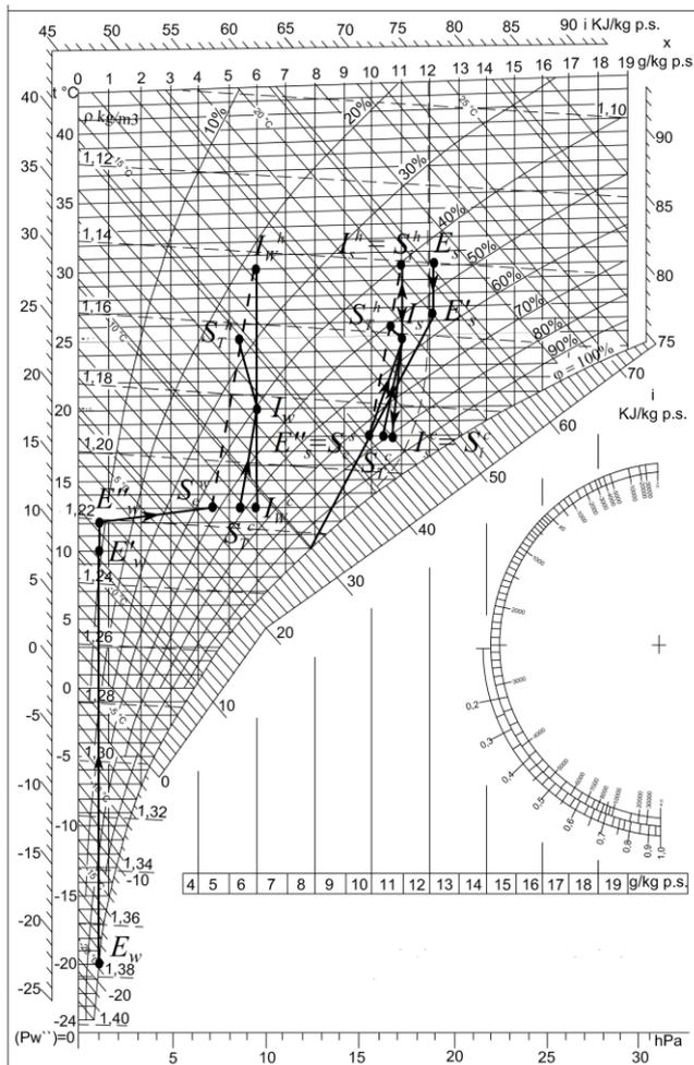
**Fig. 5.** Processes of air-conditioning airflow treatment and air transitions within a room under summer and winter design conditions for system with direct external air supply to room and cooling with dehumidification (see below for full list of symbols).
