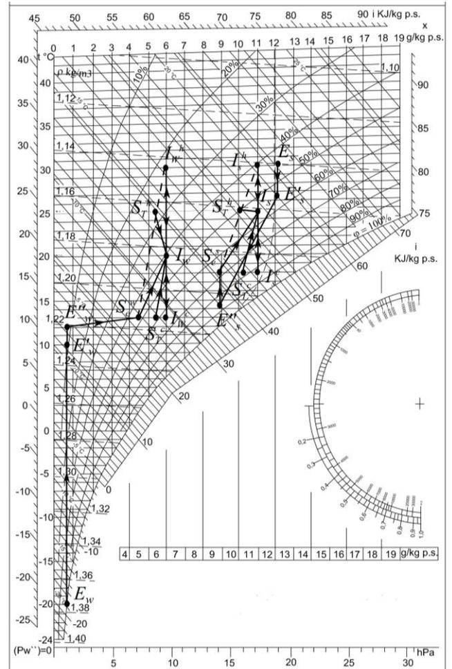
**Fig. 4.** Processes of air-conditioning airflow treatment and air transitions within a room under summer and winter design conditions for system with direct external air supply to room and cooling without dehumidification (see p.5 for full list of symbols).
