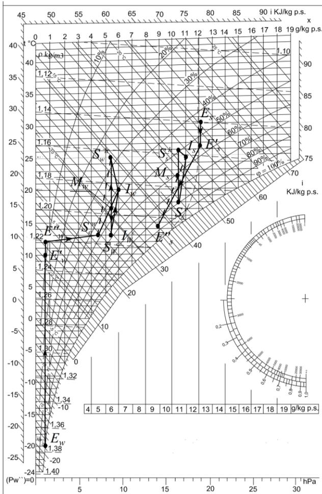
**Fig. 3.** Processes of air-conditioning airflow treatment and air transitions within a room under summer and winter design conditions for system with external air supplied to FCU suction side (see p.5 for full list of symbols).
