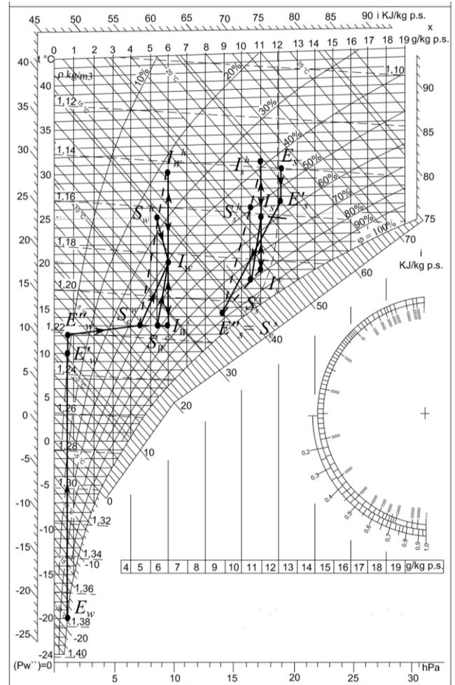
**Fig. 2.** Processes of air-conditioning airflow treatment and air transitions within a room under summer and winter design conditions for system with external air supplied to FCU discharge side (see p.5 for full list of symbols).
