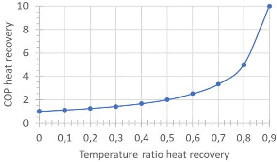
Fig. 5 : Thermal COP of a heat recovery system
