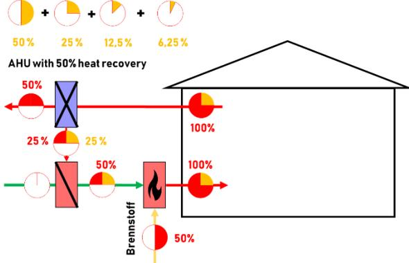
Fig. 4 : Example ventilation unit with 50% heat recovery
