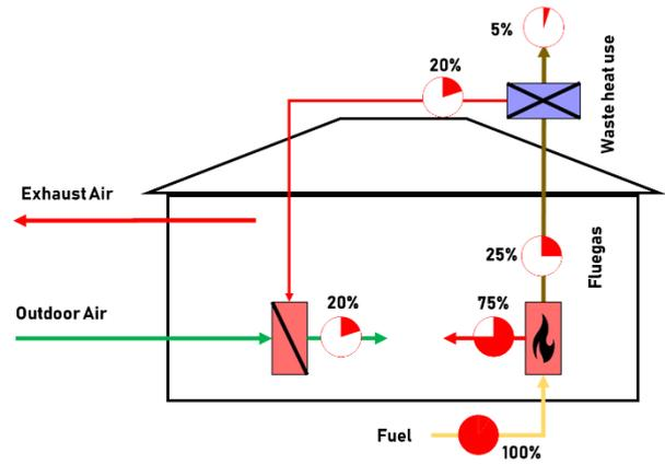
Fig. 1 : Example waste heat use with a boiler
