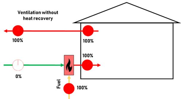
Fig. 2 : Example ventilation unit without heat recovery
