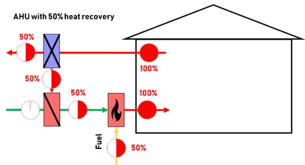
Fig. 3 : Example ventilation unit with 50% heat recovery
