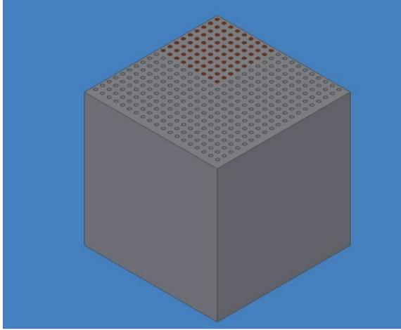
**Fig. 4.** Inserted copper tubes at equal distances
