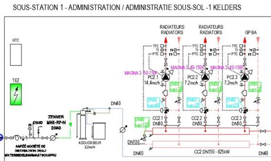
Fig. 8. Heating system diagram – substation 1
