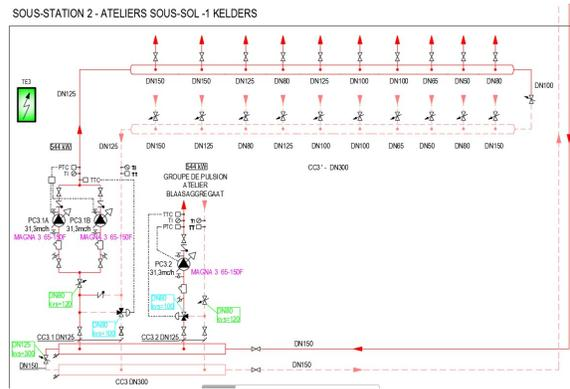
Fig. 9. Heating system diagram – substation 2
