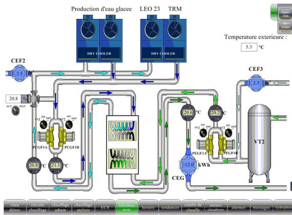
Fig. 13. Cooling system BMS diagram
