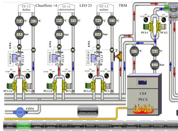
**Fig. 6.** Heating system diagram – main manifolds
