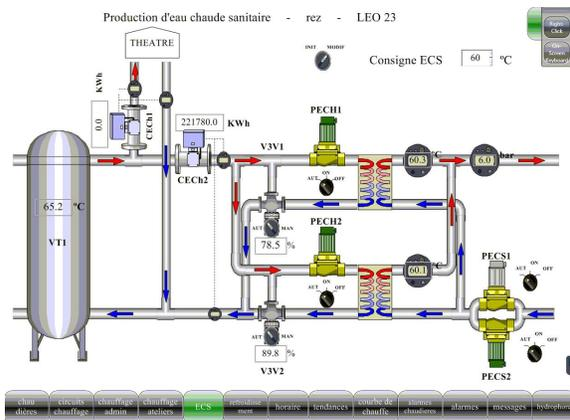
Fig. 10. Heating system diagram – domestic hot water
