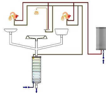
**Fig. 5.** Direct connection of the heat exchanger to several sanitary appliances (shower and two wash basins) [6]
