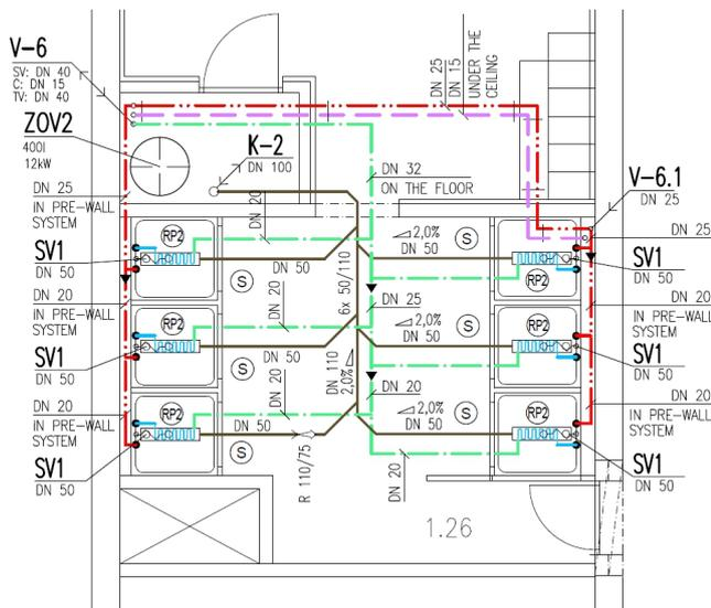
**Fig. 14.** Floor plan with alternative solution of recovery of waste heat using a heat exchanger placed under the shower tray
