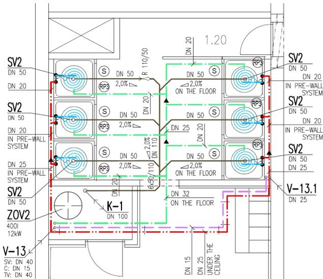
**Fig. 13.** Floor plan with alternative solution of recovery of waste heat using a shower tray with integrated heat exchanger
