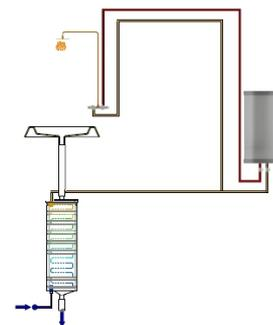
**Fig. 6.** Combined connection of the heat exchanger with a storage water heater [6]
