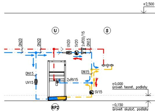
**Fig. 17.** Detail of connection of heat exchanger with bypass of cold water
