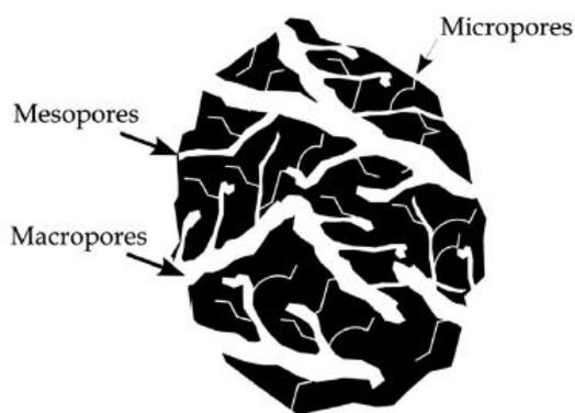
Fig. 1. Schematic representation of adsorbent pore structure [14]
