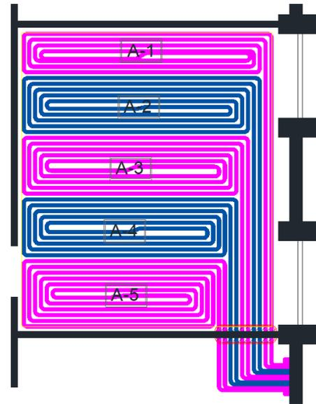
Fig. 2. Layout of the radiant floor system.
