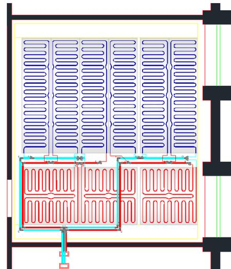
Fig. 3. Layout of the radiant ceiling system.
