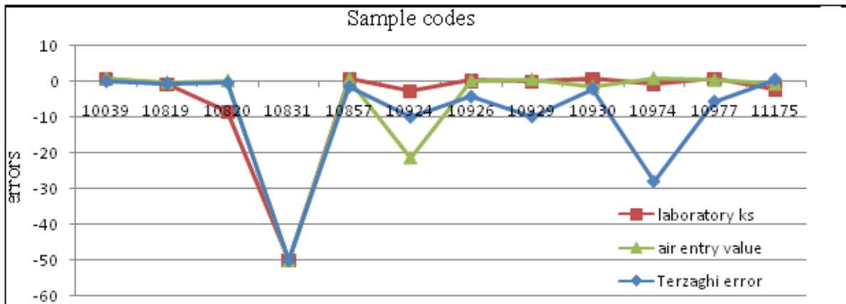
Fig. 1. Errors presented by Brooks and Corey method for a set of sand as a function of ks models (laboratory ks, air entry value, Terzaghi)
