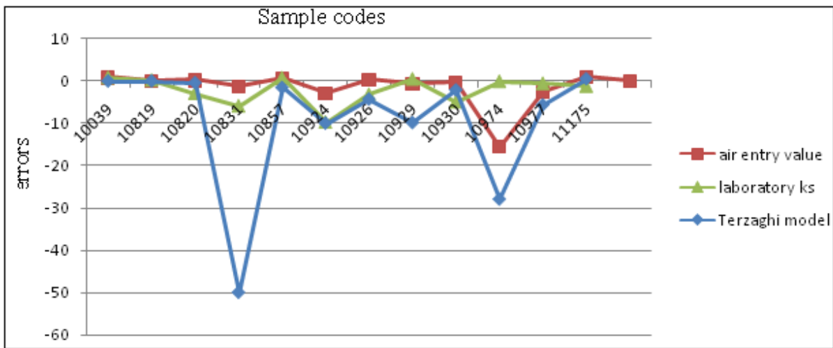
Fig. 3. Errors presented by the method of Kunze for a set of sand as a function of k_s model (laboratory k_s , air entry value, Terzaghi)
