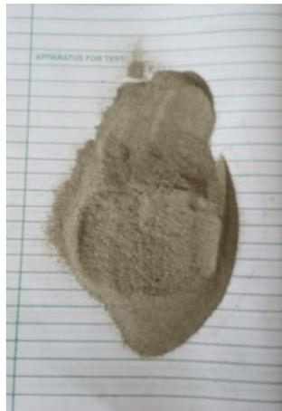
Plate 2. Sample of the pulverized PET plastic
