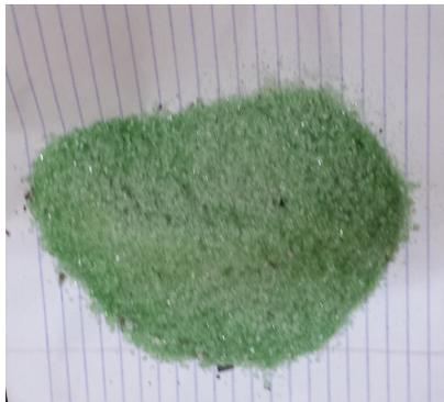
Plate 1. Sample of the recycled glass powder used in the study
