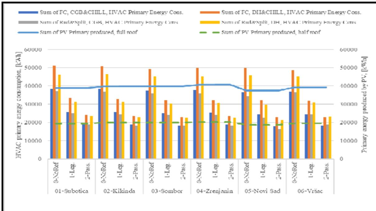
Figure 2. Comparison of primary energy consumption for space heating and cooling for various combinations and on-site produced electricity
