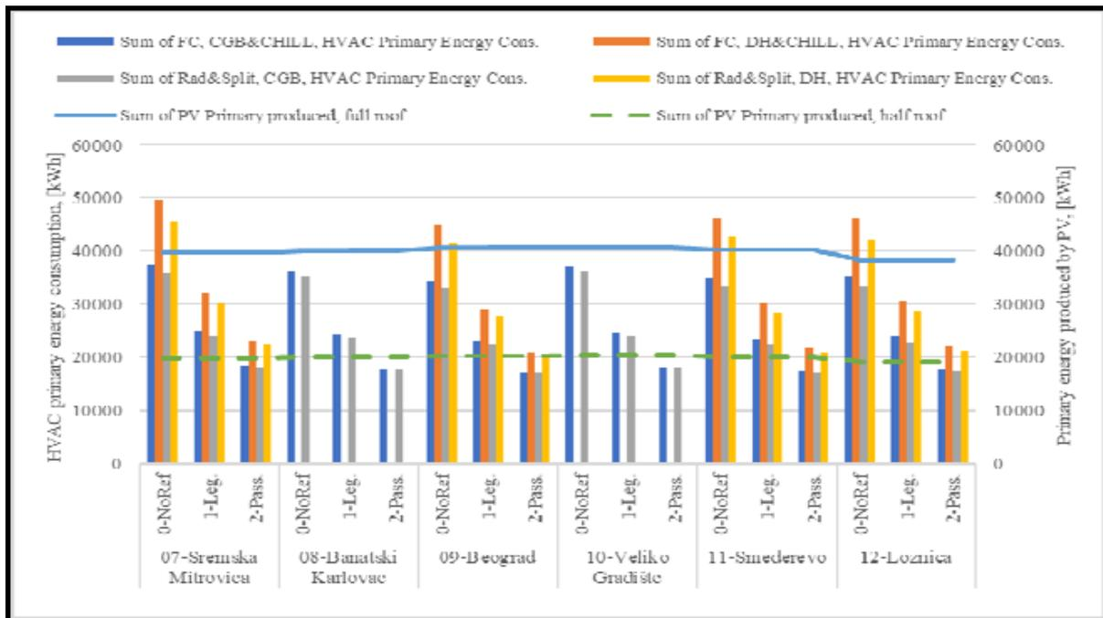
Figure 3. Comparison of primary energy consumption for space heating and cooling for various combinations and on-site produced electricity
