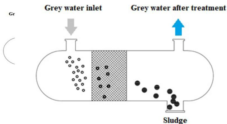
Figure 2: Schematic illustration of a horizontal coalescence filter
