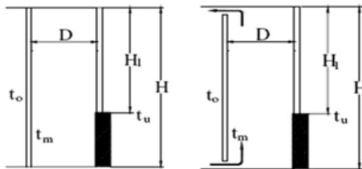
Figure 3. Double-façade constructions (left) and a wall with water flowing down
