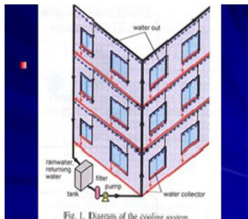
Fig. 1. Diagram of the cooling system.
