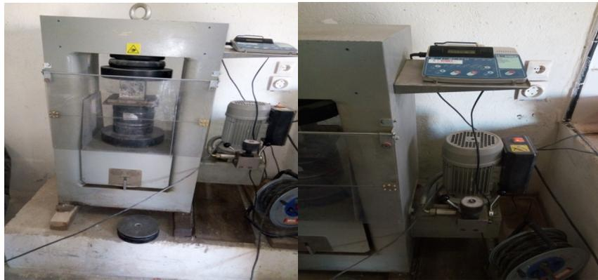
Fig.2. Machine for compressive strength test.
