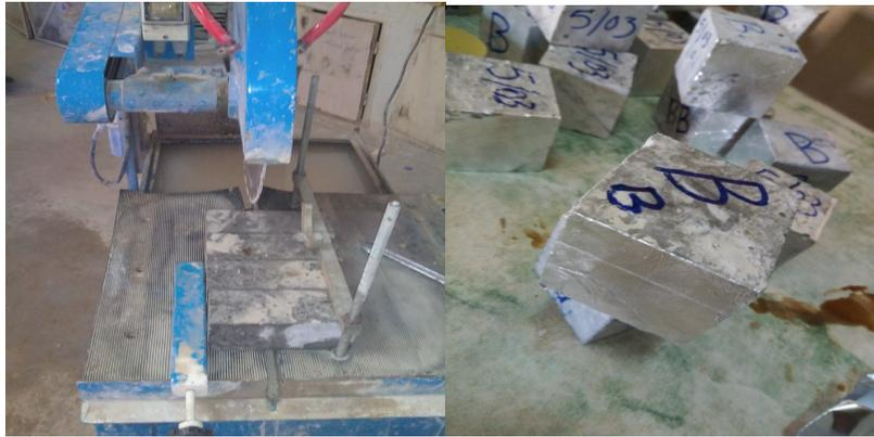
Fig. 4.: Preparation of Samples for accelerated carbonation test.
