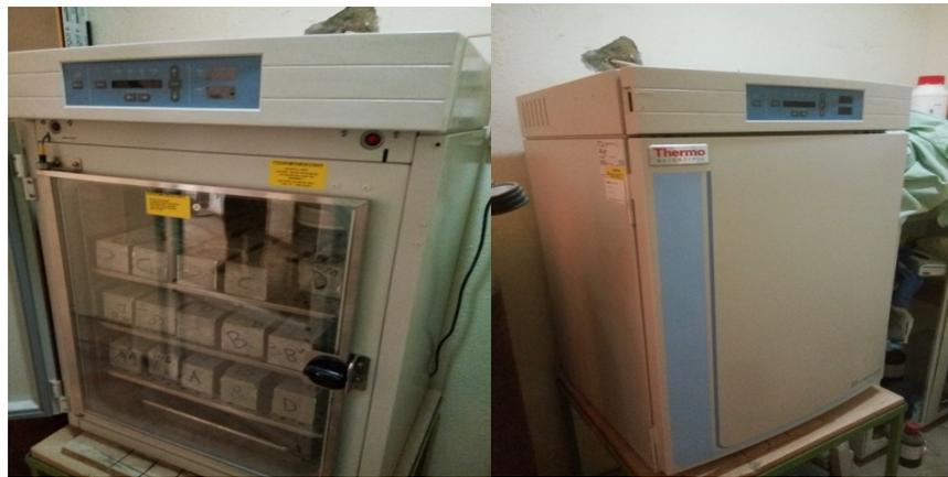
Fig.5. Samples into the chamber of carbonation
