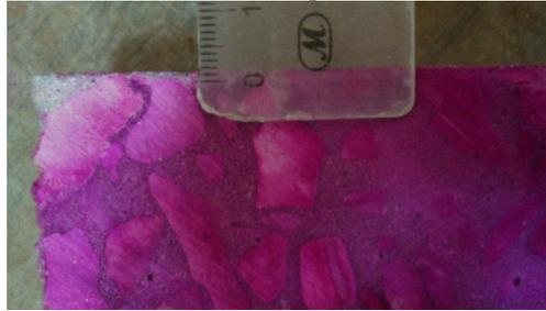
Fig.6. Determination of Carbonation depth with phenolphthalein pulverisation
