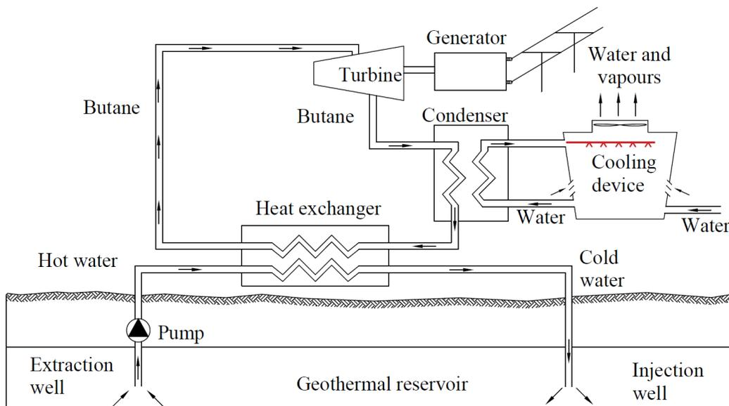
Fig. 1. Binary cycle geothermal power plant.
