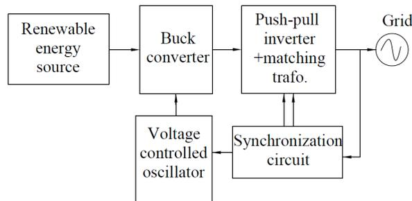
Fig. 3. Block diagram of the conversion system.
