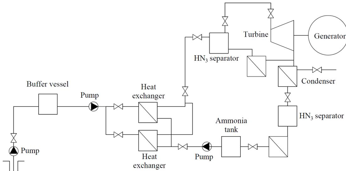
Fig. 2. Diagram of the proposed power plant.
