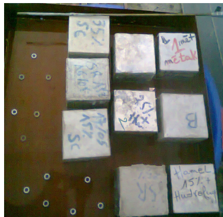
Fig.6. Water absorption test on concrete cubes
