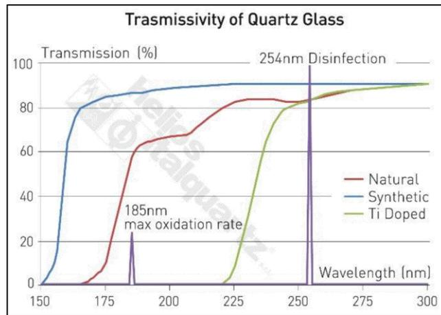
Figure 6 Different quartz glass transmissivity of UV radiation [8]
