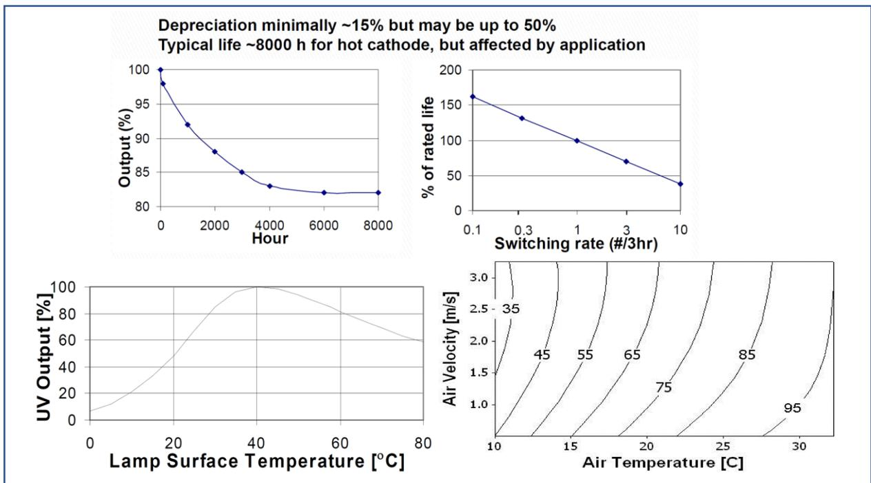
Figure 7 UV output change [%] with different parameters [10,16]
