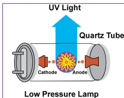
Figure 5 main operating principle of a UV-C lamp [8]
