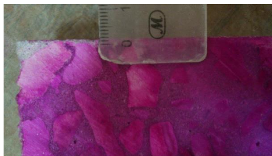
Fig.6. Determination of Carbonation depth with phenolphthalein pulverisation
