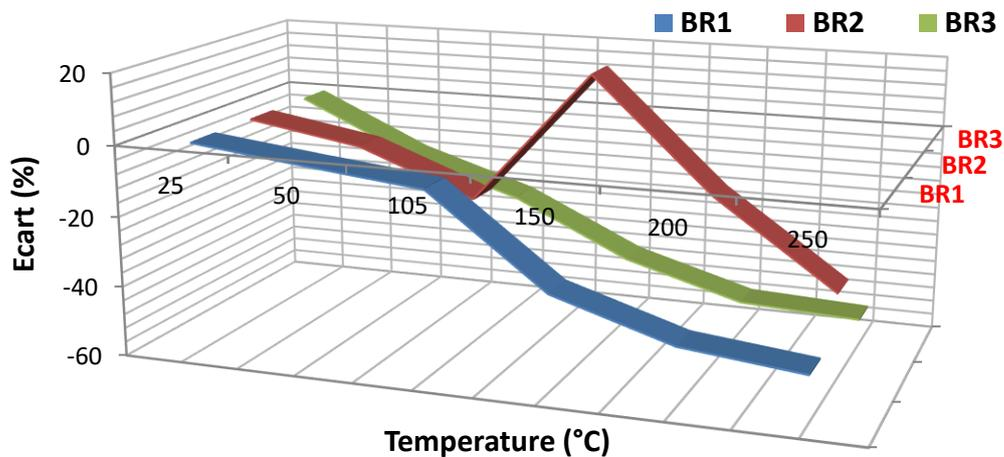
Fig. 3. Evolution of the ecart of thermal conductivity of concretes tested as a function of temperature
