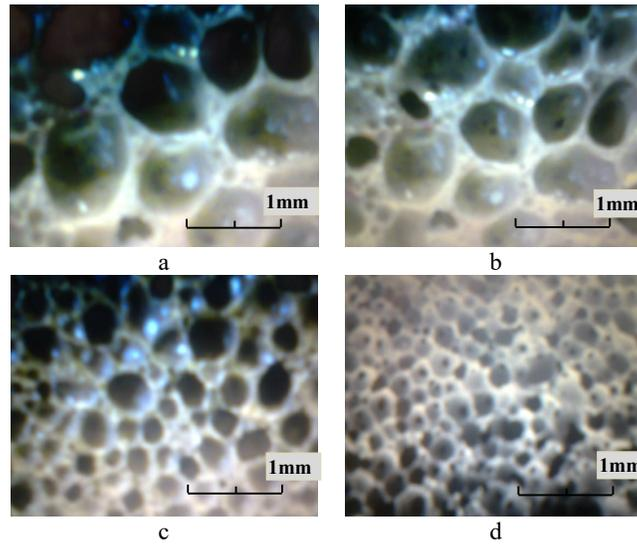
Fig. 3. Microstructural configuration of the glass foam samples
