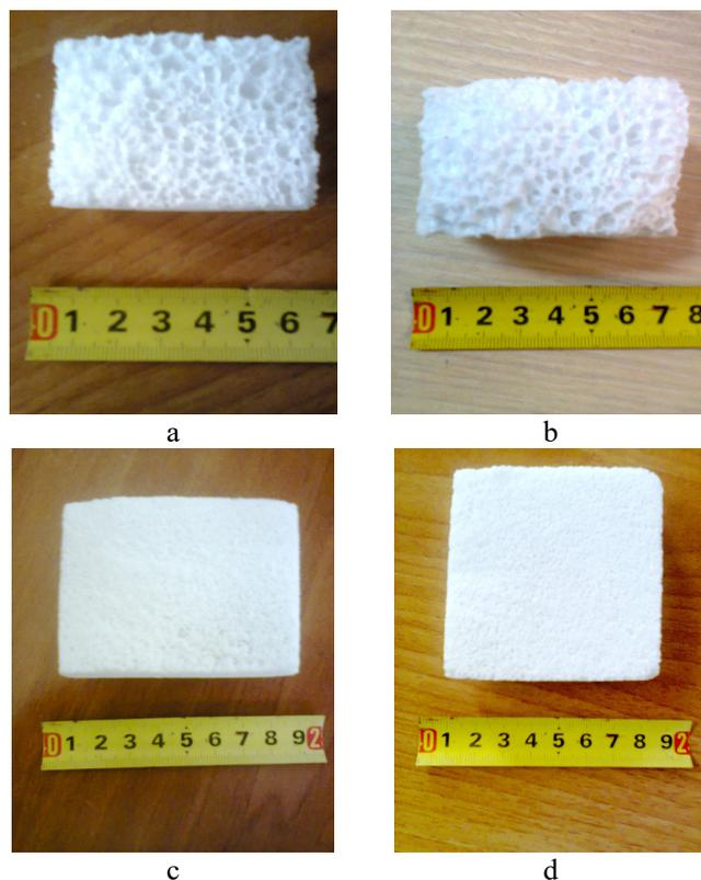
Fig. 2. Cross section of the glass foam samples
