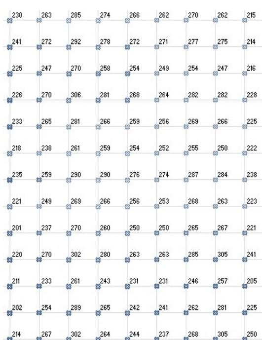
Fig. 8. Measurements in the classroom 2\*T8 fluorescent luminaire
