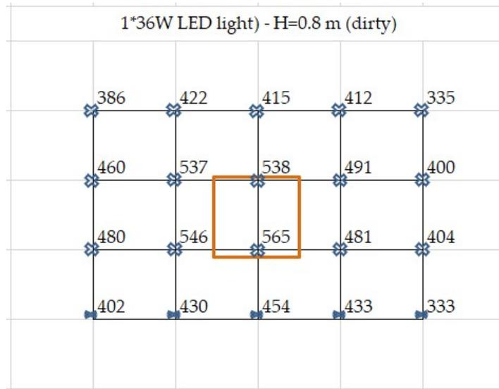
Fig. 5. Measurements LED lighting (used and dirty lamp).
