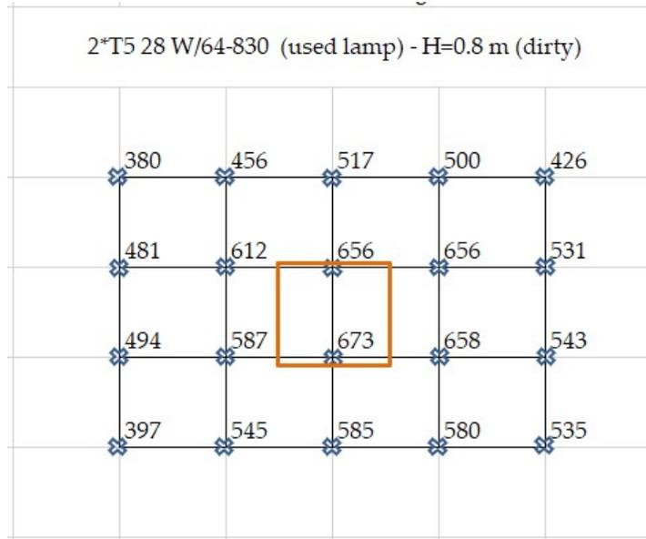
Fig. 1. Measurements 2\*T5 (used and dirty lamp).
