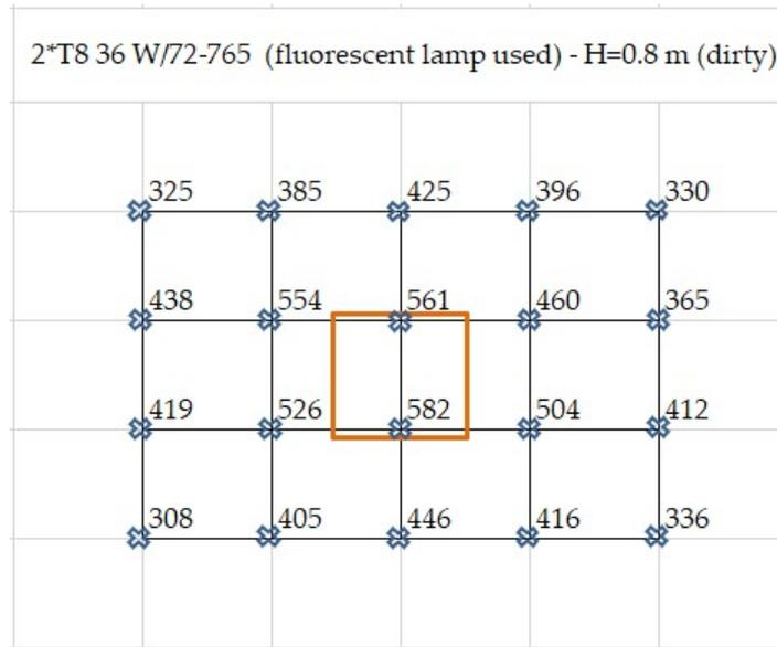
Fig. 3. Measurements 2\*T8 (used and dirty lamp).
