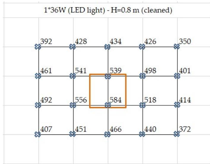
Fig. 6. Measurements LED (used and cleaned lamp).
