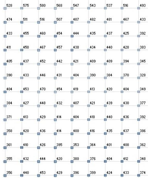
Fig. 9. Measurements in the classroom 2\*T5 fluorescent luminaire
