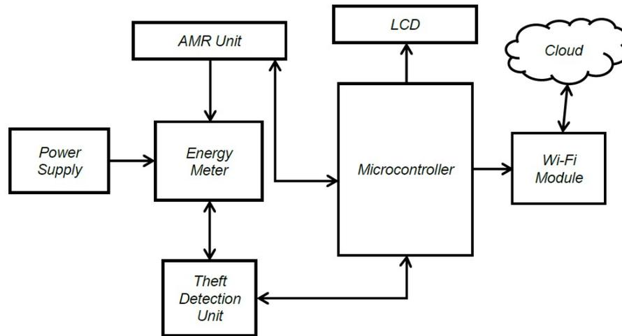
**Fig. 1** Block diagram of IoT based energy meter [7]
