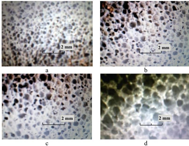
Fig. 3. Microstructural pictures of the cellular glass samples
