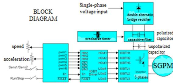
Fig. 2.2. Block diagram representation of the static converter [9]
