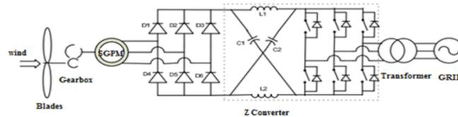
Fig.3.7 Energy conversion configuration with a Z-converter [19]
