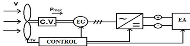
Fig 3.2. Wind system charging on electric accumulators [10]
