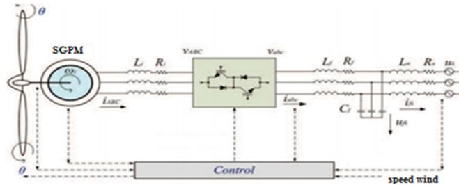
Fig. 3.5. Turbine conversion using a matrix converter [18]
