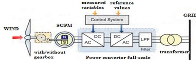
Fig. 3.1 Common model of energy conversion of a wind power plant [11]
