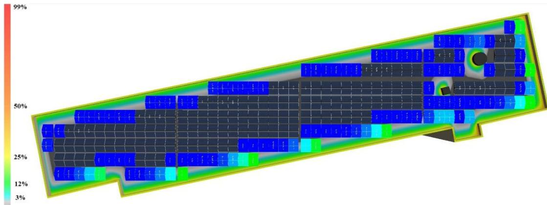
Fig. 4 Placement of PV modules on the ASPC building [1]
